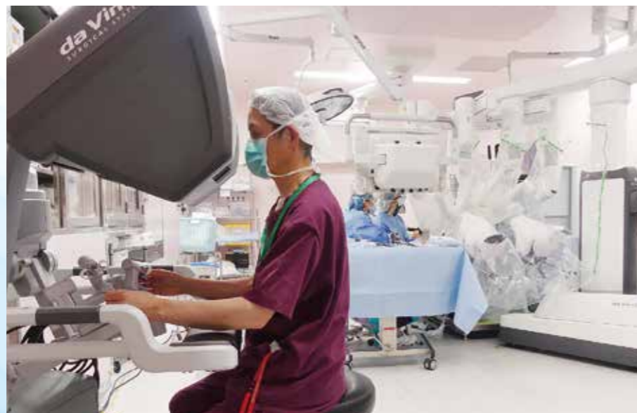
Surgery assisted by the Da Vinci surgical robot (with the operator in the foreground).
